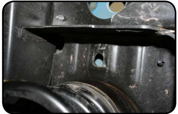
6. Using the supplied hardware, install the coil retainer in between the top to coils. Using a 3/4 socket and wrench torque the bolt to 50 Ft-lbs
