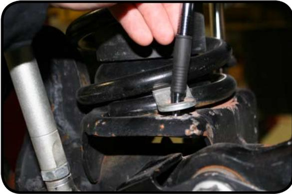
3. Drill the hole using a 3/8" drill bit.
