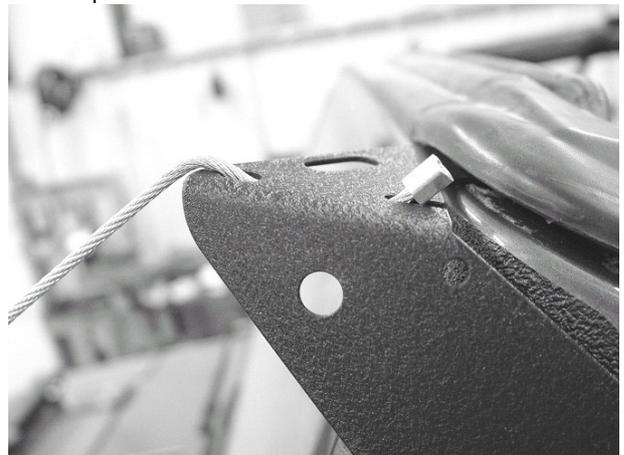
Run the threaded cable end through the hole in the fender bracket and secure with the wingnut, DO NOT over tighten.
